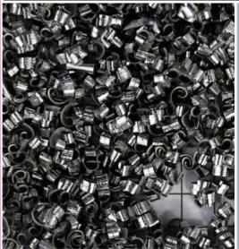
Alloy 6026<sup>LF</sup> LEAD FREE is the best option for machinability since recent limitations by RoHS (2018/740/EU) and REACH on lead content allowance (Pb  $\leq$  0.1%). It is particularly suitable for being machined on high-speed automatic lathes. 6026<sup>LF</sup> LEAD FREE offers:
